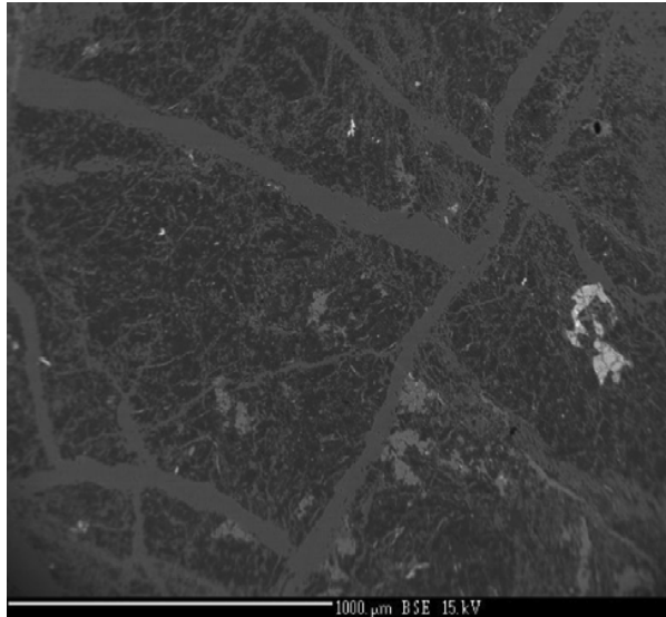
Figure 4: Back-scattered electron image of fully carbonated peridotite (listwanite), composed of magnesite (magnesium carbonate, MgCO_3 , dark grey matrix), quartz (light grey veins showing hierarchical, cross-cutting relationships, filling cracks with spacing < 100 microns) and relict chromian spinel (bright grain at right). Image from keynote talk by Prof. Peter Kelemen, Columbia University, & Streit et al., paper in prep.
